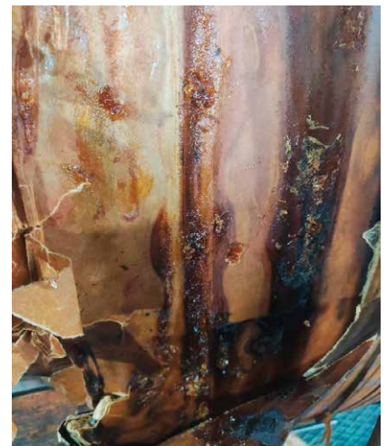
Traces found of damaged and burned glue.
