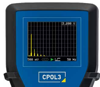
Spectrum mode (FFT) for detecting coupled signals
