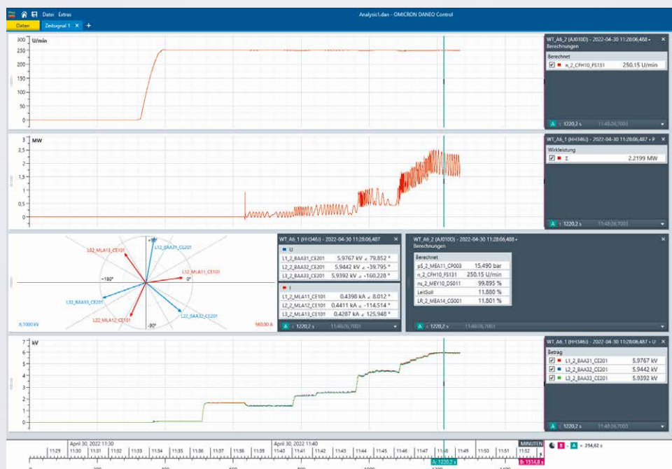
Live view of measured values in the DANEO Control
