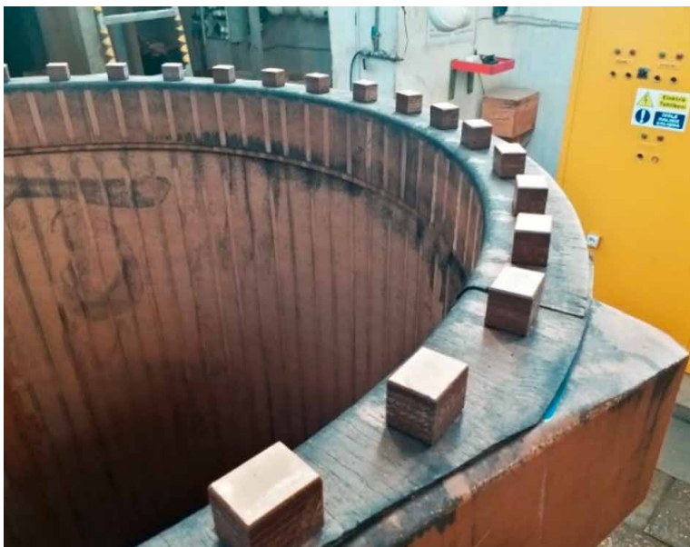
Traces of carbonization were found on various components.
